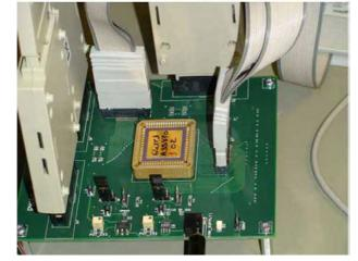
Caption: Test board and ASIC incorporating a double-memory programmable and configurable PWAG controller
