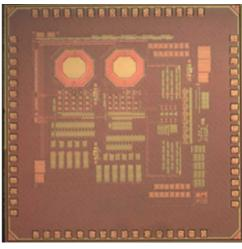
Caption: Microphotograph of a CT bandpass Sigma-Delta Modulator for RF digitization, implemented using Gm-LC circuits in a 65-nm CMOS technology
