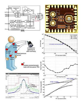
Caption: Ultra-low power transceiver for Bluetooth Low Energy (BLE). The receiver (Rx) skips any active RF stage and it is implemented as a passive front-end. It achieves a sensitivity of -81.4 dBm and consumes less than 1.1 mW. The transmitter employs direct modulation and an efficient class-E power amplifier (PA) to deliver 1.6 dBm output power to the antenna with a total efficiency of 24.5%.
