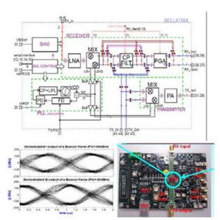
Caption: Prototype of a Zigbee/IEEE 802.15.4 transciever, implemented in a 1.2V 90nm CMOS technology
