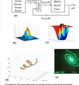
Caption: Event-driven sensing-processing system with (a) DVS-retina and multi-kernel-convolver (b,c): it captures the 500Hz oscilloscope spiral (e), generating events (x,y,t), representing the spatio-temporal trajectory (d). See ref [A] for details.
