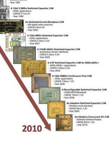
verter designed by our research group to Alcatel Microelectronics and STMicroelectronics for its incorporation into the ADSL2+ modem chipset ST20190 Utopia for CPE applications (massive production in 2004).
