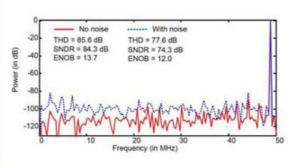
Caption: 1.8V 15-bit 100Msps Pipeline ADC: layout and post-layout simulation results of Nyquist performance with and without transient noise
