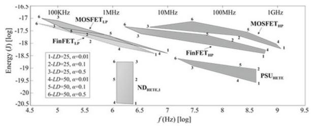
Caption: Evaluation in terms of energy and speed of CMOS transistors (MOSFETs and FinFETs) and tunel transistors (PSUHETE and NDHETE1). Different logic-deths and switching activities are explored.
