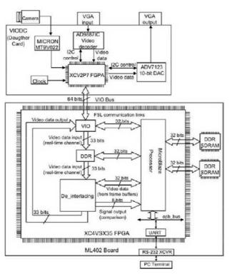
Caption: FPGA-Based Embedded System for Video De-Interlacing.
