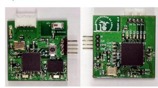
Caption: PCB developed for the leg edema test wearable system, to be applied in patients with heart fail disease. The size is set to 2x2 cm2.
