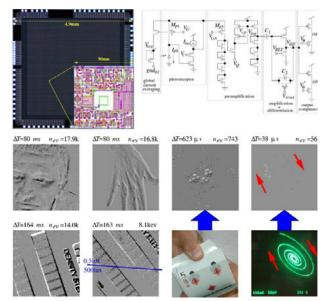
Caption: Top: DVS chip with 128x128 pixels, showing zoom preview of  $30\mu m$  size pixel and schematic on the right, fabricated in AMS 0.35 $\mu m$ . Bottom: Example captures of DVS camera showing high-speed capability, low data-rate (nev is number of events), high intra-scene dynamic range. See ref [A] for details.
