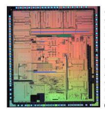
Caption: Photograph of ASIC CMOS 0.35µm Front-End for solar irradiation sensors on the surface of Mars. The circuit has been designed with the radhard library (hardened against radiations) developed at the Microelectronics Institute of Seville (IMSE-CSIC-US).
