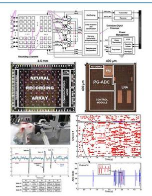
Caption: Fully implantable multichannel cortical neural recording system and experimental verification in vivo with animal model.
