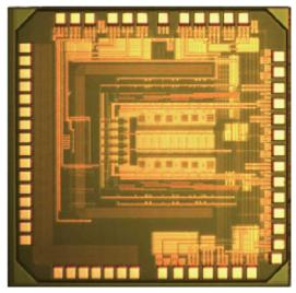
Caption: Microphotograph of a programmable SC lowpass cascade Sigma-Delta Modulator for SDR applications, implemented in a 90-nm CMOS technologyModulator for RF digitization, implemented using Gm-LC circuits in a 65-nm CMOS technology
