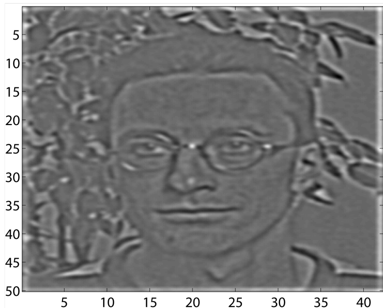
Figure 8.26: The image of figure 8.23 that has been convolved with a 'difference of Gaussians' convolution kernel: Local contrast, mostly edges, are enhanced. Uniform surfaces appear gray.
