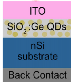
Figure 3.22: Schematic view of a Ge QDPD on a silicon substrate [5].
